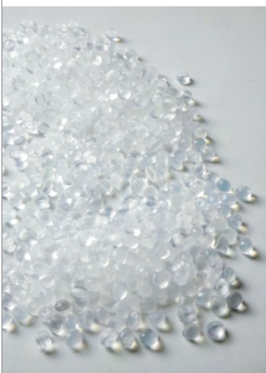
The plant uses ethane derived from the nearby Marcellus Shale to produce polyethylene, one of the most common thermoplastics.
