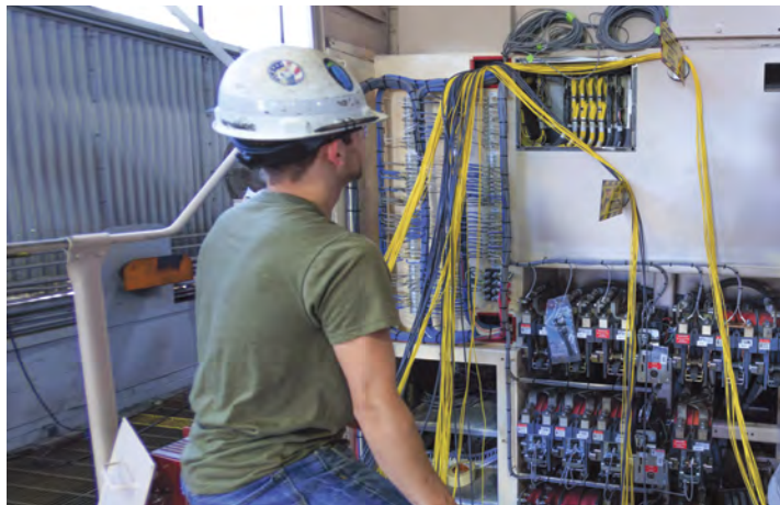
IBEW electricians from Huntington, W.Va., Local 549, like Chance Brown, above, are part of a unique team of union workers at CSX who are stripping as many as seven diesel-fueled locomotives a year down to their frames and then using recycled and modernized components to rebuild them as hydrogen-powered engines.
