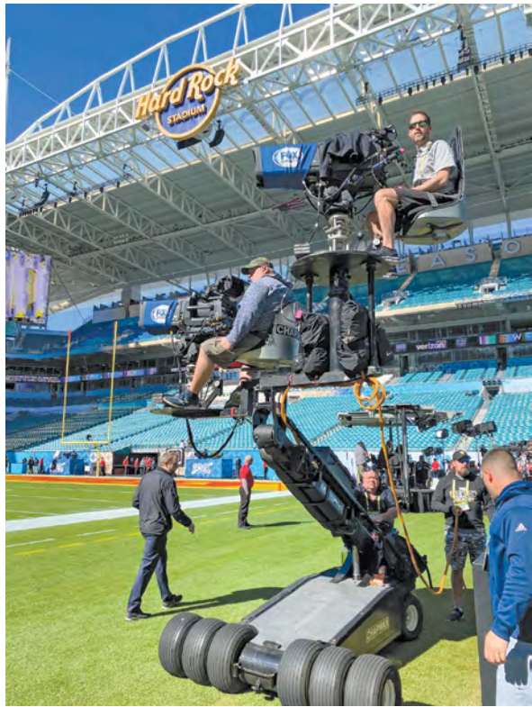
New York 1212 members Matt McGahan, top, and Mario Zecca operate the Chapman camera crane, which allows for camera shots above the players on the sideline, during Super Bowl 54. The pair were a part of a 400-person Fox Sports crew.
