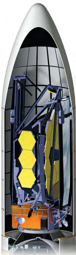
*The largest space telescope in history, the Webb telescope will fold up to fit the launch capsule.*
