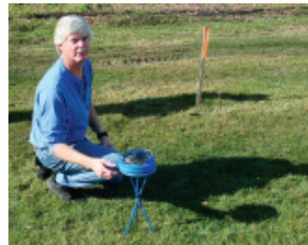
Local 673 member and JATC Instructor Ken Farabaugh demonstrates to his Solar Photovoltaic class how to set up the Sun Path Calculator, used to evaluate shading at potential array locations.
