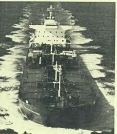
G T Chevron Oregon sailing full speed under full ballast condition during sea trials.
