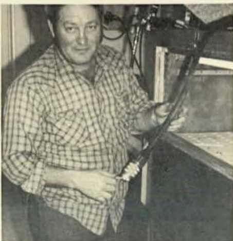
Jim "Zero" Hays showing a plug connector that he has just removed from potting mold. Jim had to complete a NASA approved course to learn this skill and to certify.
