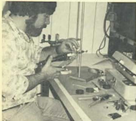
Steve Sullens using a crimp tool for terminating a crimped pin type of plug connector.
