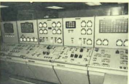
Ship control center alarms and controls for ships operations and propulsion systems are contained in this panel.
