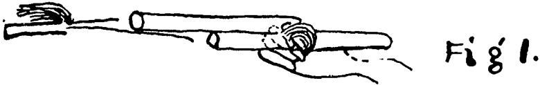
By turning the tubes they will very easily slip over the paper insulation.
